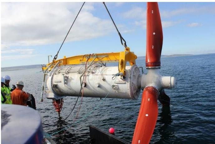
Andritz Hydro Mk1 1.5 MW Sea-Bed Mounted Turbine
